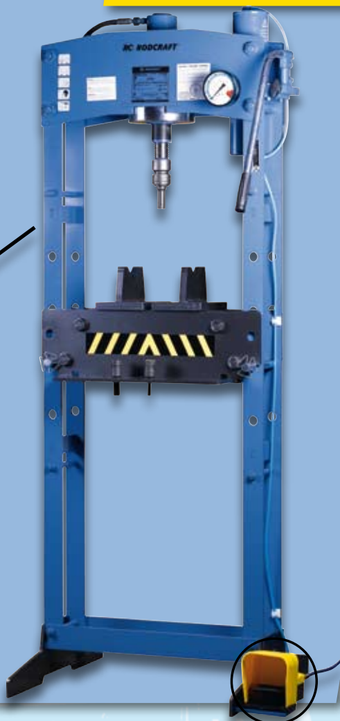
with pedal-activated air-hydraulic pump
