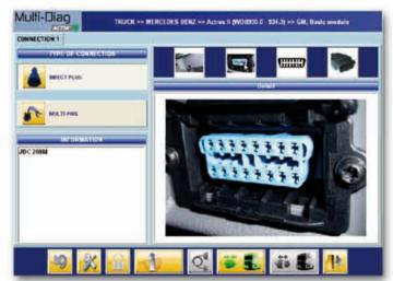
4. Multi-Diag® Trucks shows you where the diagnostics plug is located and the right cable to connect to the vehicle.
