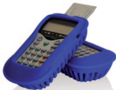
SmarTach® D-Box "All in one" tool for downloading tachograph and smartcard data.
